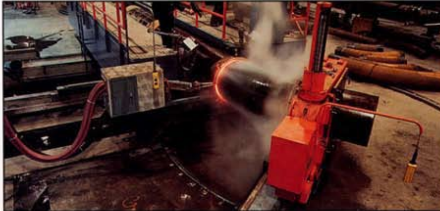
The induction bending process in operation at Indutech.
