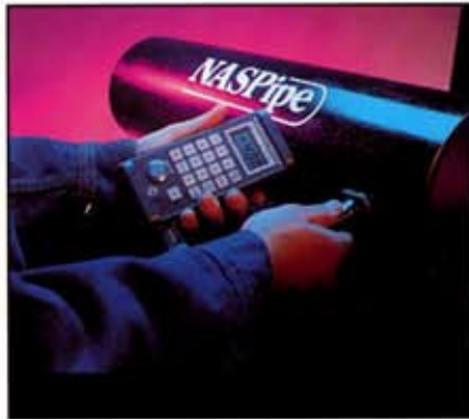
NASPipe's monolithic structure facilitates in service ultrasonic measurement of wall thickness.
