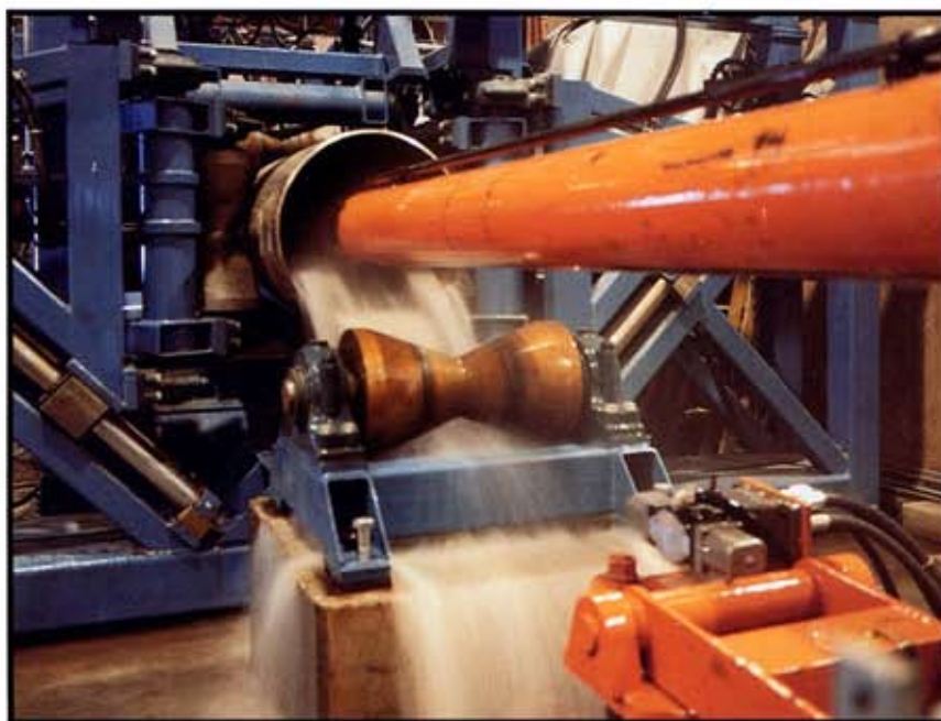
24" diameter pipe leaving the induction heat treatment machine.
